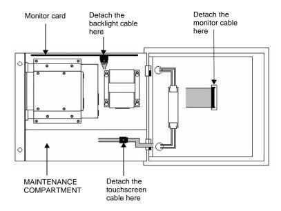
a. Detach the monitor (ribbon) cable from its connection at the center of the monitor frame (push back the locking clamps from either side of the connector).
