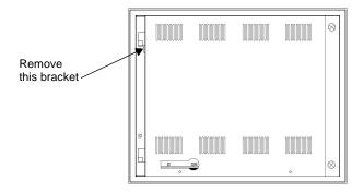
8. Lift the backshell off its hinges, and place it on a static dissipative mat in a location free from dirt and moisture and protected against static discharge. You may leave the faceplate mounted in the enclosure.
