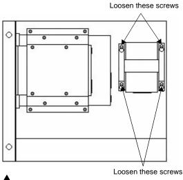
Slide the hard drive assembly up and out of the unit
