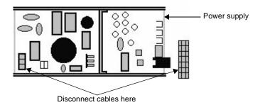
**Important** Each set of cables is gathered in a cable harness, and each harness has a plastic tab that you must pull back in order to detach the harness.
