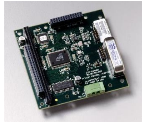
MachineLogic's Soft Runtime solution includes a Control Adapter Card, for fail-safe features such as retentive memory, watchdog timer and power fail detection.
