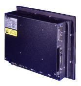
The new addition to the P1 PowerStation line features a 10", Pentium 166 processor package. Like the other P1 products, this new economical 10" unit is available with a color or mono display option with PC/104 expansion. The P1-10" comes bundled with Interact core modules (panel tools, graphics, alarming, and networking), and can also be bundled with any of the Interact optional modules, as well as MachineLogic, CTC's PC-Based Control Software.
