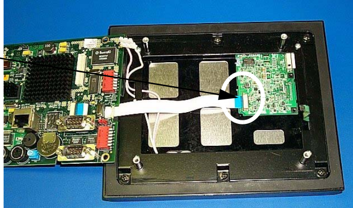
Figure 7b: Accessing the Video Cable on the BZK-08T5
