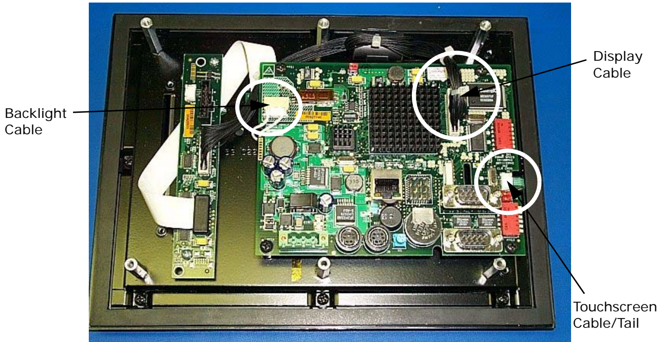
Figure 4: Accessing the BZK-08T1 Internal Cables
