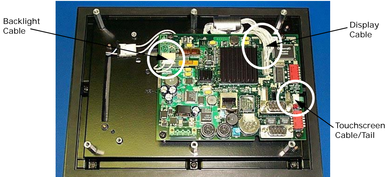
Figure 4: Accessing the BZK-08T1 Internal Cables
