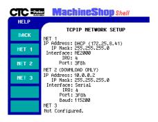
The display area of the screen shows the current network connection settings. Specific settings for each connection are based on the installed Network Interface Cards.
