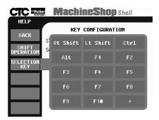
4. Choose a keyboard key from the submenu. The Select key on the P5 PowerStation faceplate will act like the key you have chosen, while you are in Interact. The following selections are available: Right Shift (default), Left Shift, Ctrl, Alt, F1 through F10, and Keypad +.
