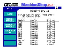
The Shell automatically scans and detects if a security key is attached to the workstation. If a key is detected, the display area shows the serial and key number, the Interact modules, and the features that are enabled in the "Runtime Key". The display area also lists the module's acronym followed by its status which can be Runtime, Config, or Transferred.
