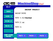
2. Select one of the PATH submenu buttons (1,2, or 3). The backup path entry screen appears.
