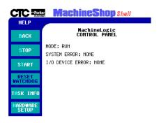
The display area of the screen shows the current mode (STOP, RUN, or HALT) of the MachineLogic runtime. It also displays error information. If an error condition occurs, the error number and the corresponding message will be displayed on the screen.
