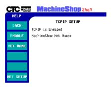
Note Changes made to the TCP/IP Settings are written to the TCPIP.INI file located in the NET directory. Changes do not take effect until the runtime workstation reboots. A confirmation message will display when you exit the TCP/IP Setup screen asking if you wish to reboot the system.
