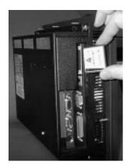
3. Insert the CF card into the PC's PCMCIA slot, using the CF-to-PCM-CIA adapter.
