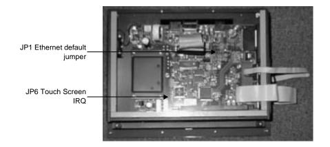
**Note** The PowerStation's CPU card also has several sets of jumpers that may also be changed. Refer to the CPU manual that came with your PowerStation for more information about changing these jumpers.
