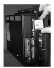
3. Insert the CF card into the PC's PCMCIA slot, using the CF-to-PCM-CIA adapter.
