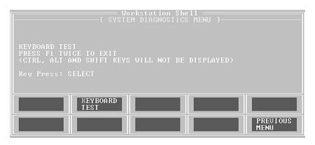
**Note** If your PowerStation has a touch screen, upon pressing the display the text string "SELECT" is displayed. Also, pressing the Shift, Ctrl, and Alt keys does not display a text string.
