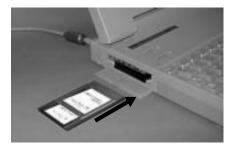
The PCMCIA drivers should recognize and configure the card as an ATA card, assigning an additional drive letter for the card (e.g., D:)
