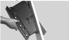
3. Remove the back cover by removing the 5 screws shown below.
