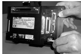
Figure 2-1: Connecting an Ethernet Cable to Motion-Panel
