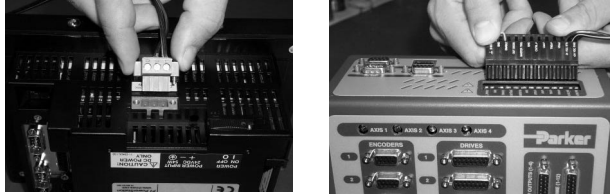
Figure 2-3: Connecting Power to MotionPanel and the Controller
