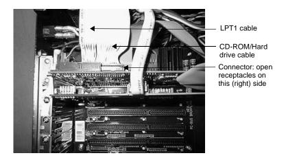
**Note** You may need to disconnect the LPT1 cable from the card first in order to connect the hard drive or CD-ROM cable.
