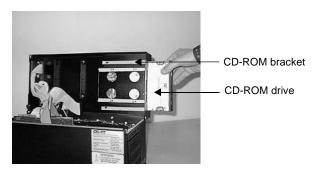
3. Fasten the drive in place with the four retaining screws included in the installation kit.
