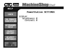
3. On the **PowerStation Settings** submenu, press the **Calibrate Touchscrn** button.
