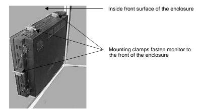
3. Tighten each screw against the front of the enclosure to a torque of 0.5 lb./in.
