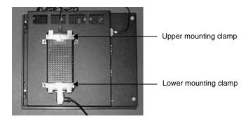
4. Fasten the adapter to the monitor with the four retaining screws included in the adapter installation kit. The completed installation should look like the illustration below.
