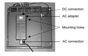
3. Place the two adapter mounting clamps over the top and bottom of the adapter, as shown below. Align the holes in the clamps with the mounting holes in the back of the monitor.
