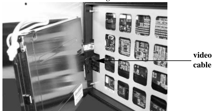
Figure 4 Disconnecting the Video Cable
