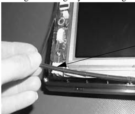
Figure 6 Securing the Rubber Gasket
